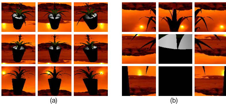
Figure 13. a) Perspective images from different views, (b) example of a hogel image.
