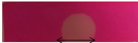
Figure 6. 3. Imaged Layer containing TEA initiator composition 'A' exposed to laser 532nm wavelength
