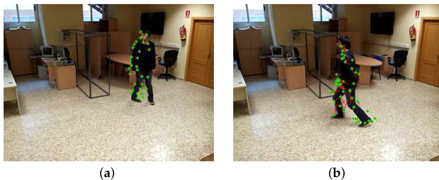
Figure 8. Optical flow applied to the subject in a scene. (a) Subject rotating. (b) Subject getting up after a fall event.
