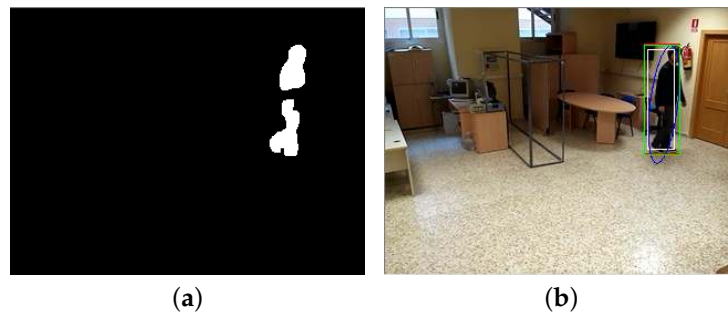
Figure 6. Broken contour reconstruction example. (a) image with separated contours; (b) image with reconstructed contour.
