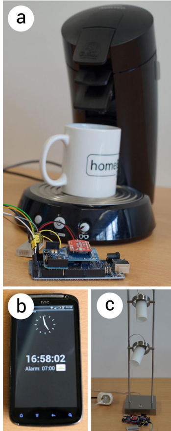
Figure 4: homeBLOX smart devices: (a) smart coffee maker, (b) UPnP alarm clock, and (c) smart lamp.
