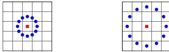
Figure 4.5: The figure indicates the support adopted by all three local operators. The application pixel is denoted with a square and its neighbors are indicated with circles. The left panel shows the operator with support parameters ( r = 1, n = 12 ); the right panel displays the operator with support parameters ( r = 2, n = 12 ).
