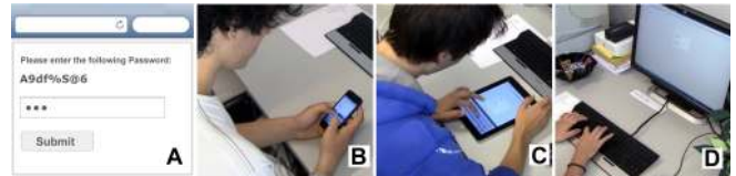
Figure 1. In the pre-study, input performance was assessed on an Apple iPhone 5 (B), an Apple iPad 4 (C) and a Desktop PC (D). The same graphical user interface (A) was used on all devices, but adjusted to fit the respective screen size.
