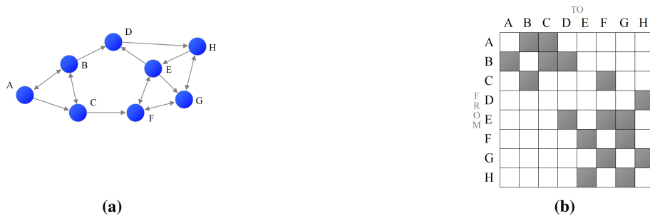
Fig. 1. Social network visualizations. (a) A node link representation of a very simple 8 node network (b) An adjacency matrix representation of the same network, note that the number of grey cells is equal to the number of links in (a)
