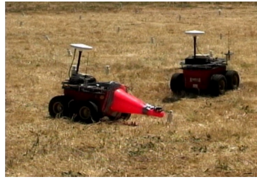
Figure 7: Object tracking applications. left) Indoor testbed with 25 nodes. An RC car and a pan/tilt camera. As the remote control car is driven through the sensor field, the network locates the car and sends the position to the camera, which visually tracks the vehicle. right) Real outdoor deployment with 100 nodes and two robots. As one robot moves, the network reports its position to the second robot (with the safety cone), which pursues it autonomously.
