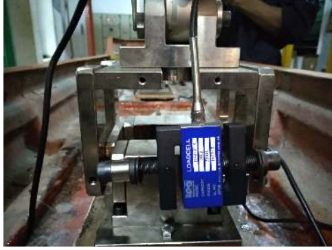
FIGURE 12. loadcell mounting arrangement: actual setup
