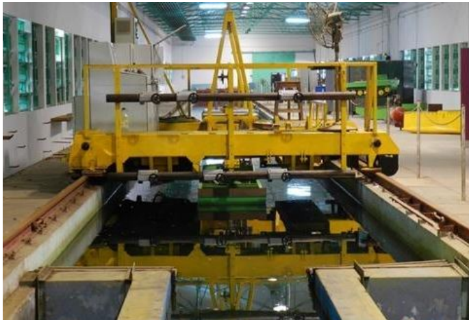
FIGURE 1. Towing Tank and Carriage
