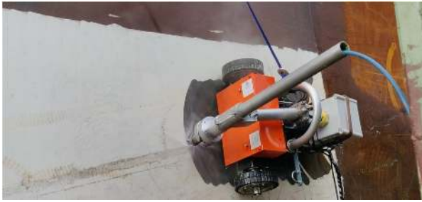
Figure 9: Hornbill robot while performing paint stripping process
