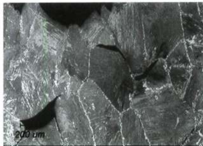
Fig. 4—Typical optical micrograph showing thin films of ferrite decorating the prior austenite boundaries, Nb steel, test temperature, 800 °C.
