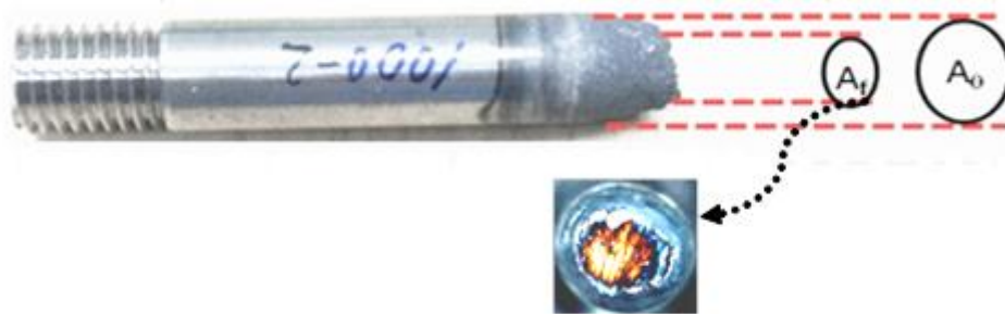
Fig.3.9 Geometry of sample after fracture.
