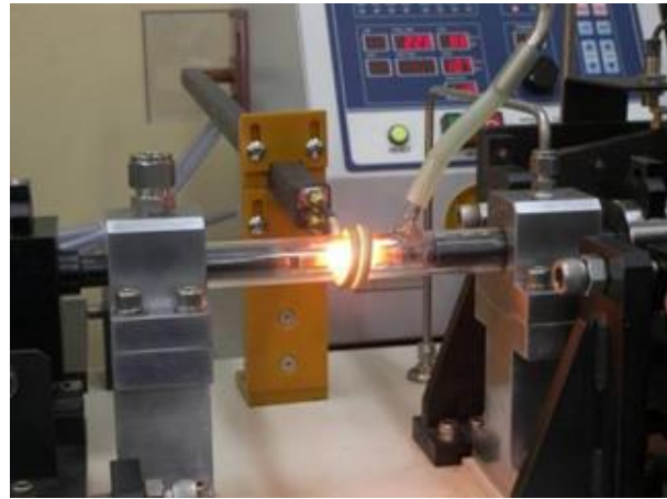
(b) heating by induction heater
