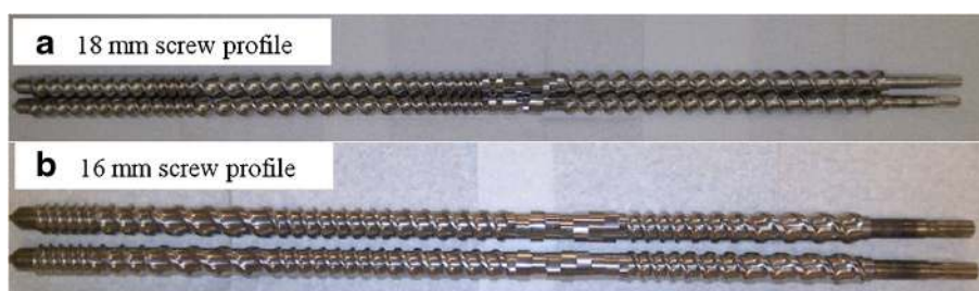
Fig. 1. Screw profile of Leistritz's a micro 18-mm and b nano 16-mm extruder
