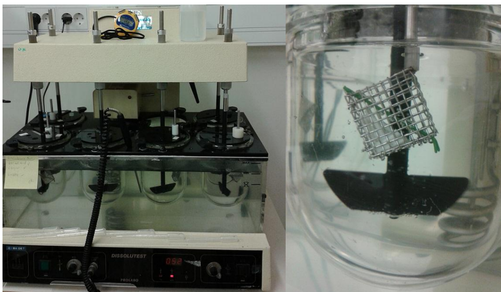
Figure 16. The experimental setup for dissolution testing: USP paddle apparatus (left) and basket with pellets submerged in dissolution medium (right).
