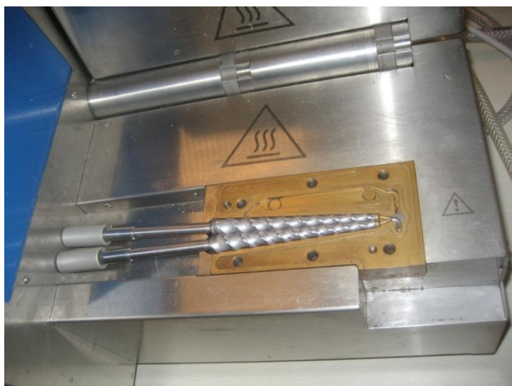
Figure 15. Haake Minilab extruder with co-rotating twin-screws.
