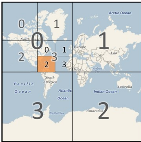
Figure 6. The tile pyramid. Tile 032 (highlighted) is at location x=2 , y=3 , level=3, and is one-fourth the size of tile 0 in each dimension.
