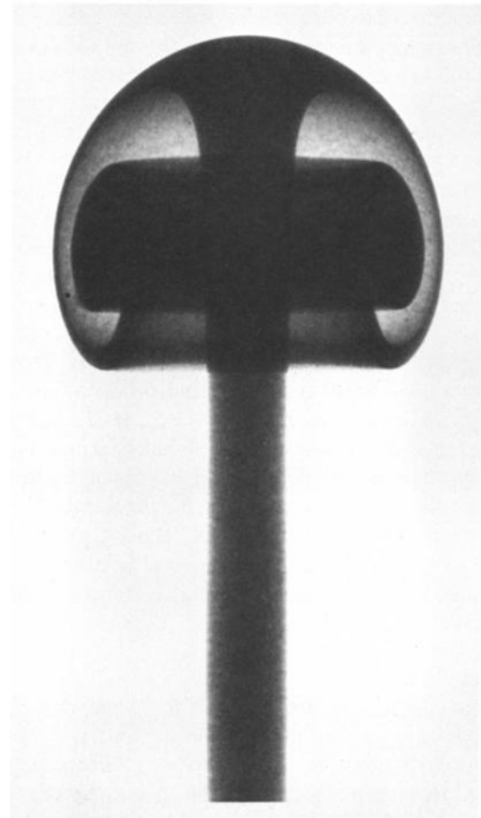
Figure 13b. Photograph of a starting thermal plume formed by injection of hot, dyed glucose into a tank of cooler, clear glucose [from Griffiths and Campbell, 1990].
