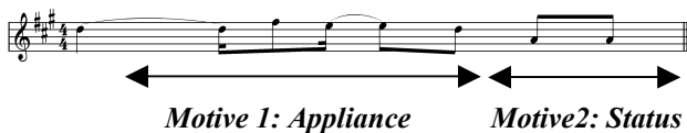
Figure 2. Earcon design. Motive 1 represents the appliance, Motive 2 represents the status (e.g. on/off). The sequence of the 2 motives indicate the status of the appliance at the moment.
