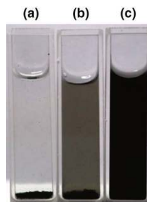
Fig. 22 Suspensions of 1 \text{ mg mL}^{-1} sulfur composites dispersed in a SA; b CMC; c LA132 after an overnight settlement. Reproduced with permission from Ref. [175]. Copyright 2016 Elsevier
