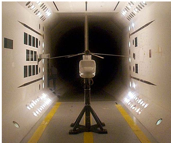
Figure 4. The ARES testbed in the TDT with the ATR prototype blade hardware installed.
