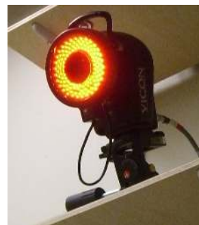
Figure 1. VICON motion capture camera. Lens located at center of the LED-array.
