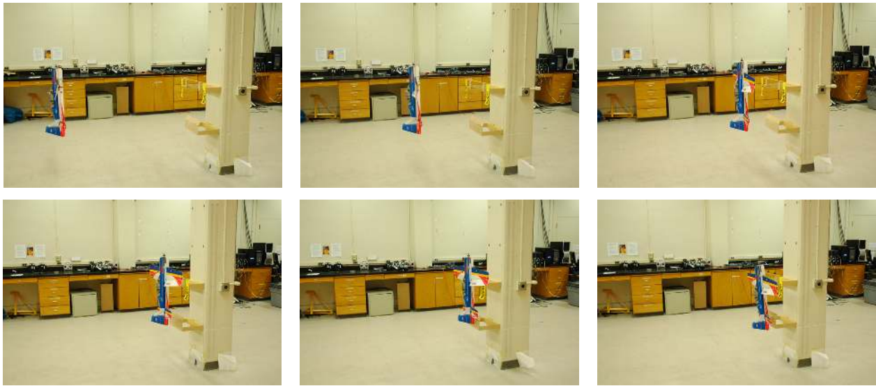
Figure 6. Autonomous landing in hover mode – perching on the fixed landing platform on a pole
