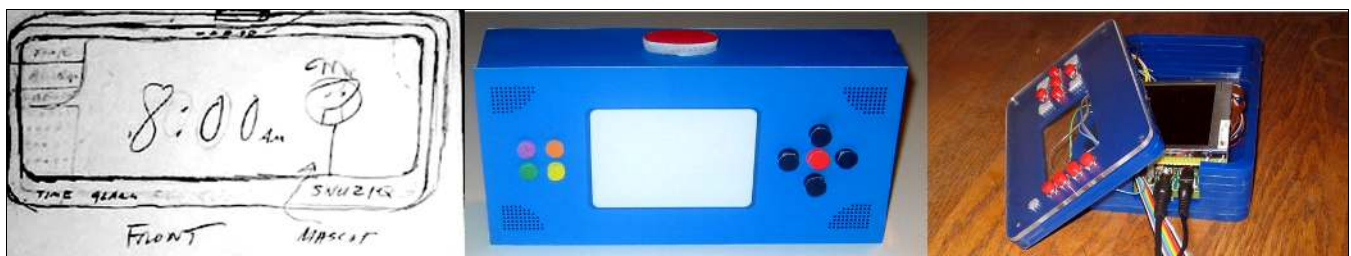
Figure 3 A paper sketch, physical mock-up, and final prototype, showing how the interface of SnuzieQ, an alarm clock, evolved through prototyping.
