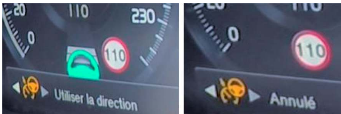
Fig. 5 Visual display of the V90 for hands on wheel required and system de-activated (Photos copyright UTAC CERAM and FONDATION MAIF)
