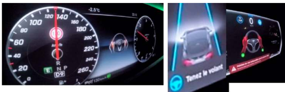
Fig. 6 Visual interface of the Mercedes E (left) and the Tesla Model S (right) (Photos copyright UTAC CERAM and FONDATION MAIF)
