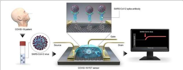
**Fig. 4** Schematic diagram of COVID-19 FET sensor operation procedure. Graphene as a sensing material is selected, and SARS-CoV-2 spike antibody is conjugated onto the graphene sheet via 1-pyrenebutyric acid N-hydroxysuccinimide ester, which is an interfacing molecule as a probe linker (Reprinted with permission from Seo et al. [118])
