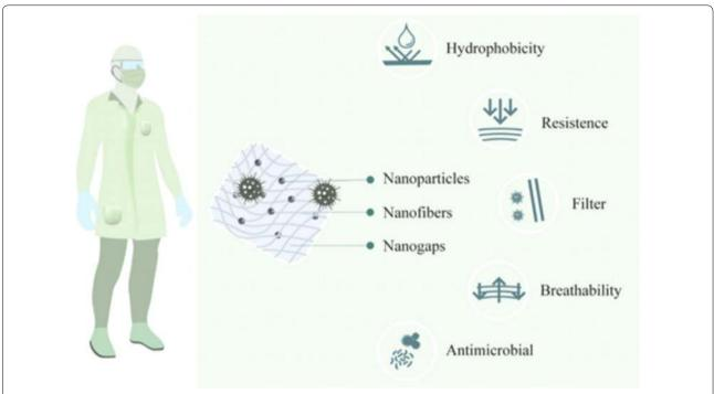
Fig. 2 Nanotechnology applications for production of PPEs. The use of nanomaterials can give new properties making the materials more resistant, efficacious, comfortable and safer for use
