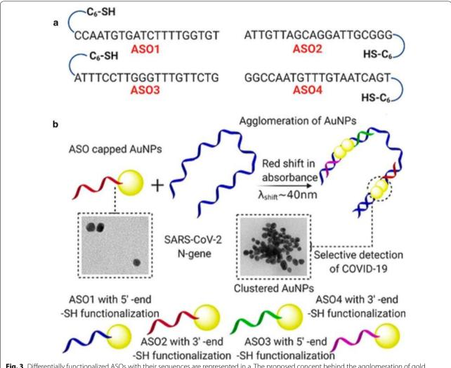
**Fig. 3** Differentially functionalized ASOs with their sequences are represented in a. The proposed concept behind the agglomeration of gold nanoparticles, when capped with the ASOs, is schematically presented in **b** (Reprinted with permission from Moitra et al. [109])
