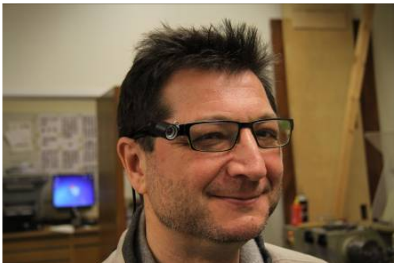
Figure 2 : subject wearing a subcam ('light' version, 2010): the camera is attached to the subject's own glasses (small black cylinder). Wire goes behind ear to wearable recorder
