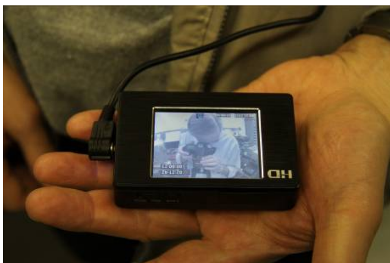
Figure 3 : Subcam, 2010 version, the recorder (carried in a pocket or clipped to belt). Wire goes to camera head.
