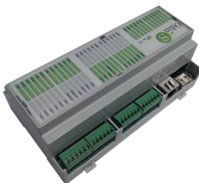
Figure 7. Home automation module developed.
