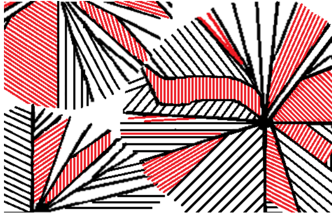
Figure 14. A schematic (not to scale) model of the possible double crystalline lamellar stacking morphology inside mixed spherulites of the BS 45 BAz 55 38 copolymer at -30°C. The black lines indicate PBS-rich lamellae while the red lines correspond to PBAz lamellae.
