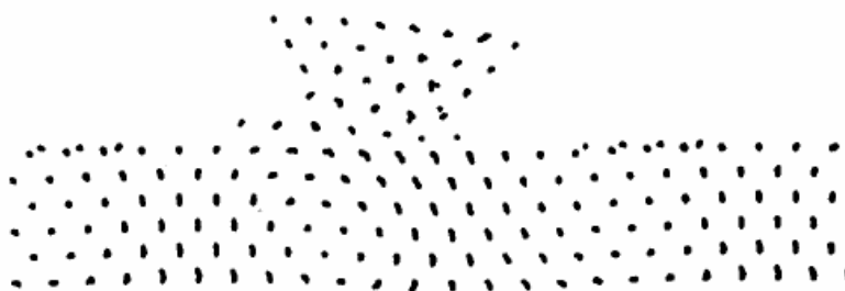
The bending of the tip under sliding shear stress. This schematic diagram corresponds to fig. 4 (c), shown enlarged below.
