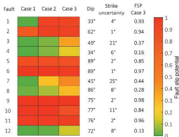
Figure 8. FSP after Walsh and Zoback (2016) for faults derived from hypocenter locations for different assumptions of the accuracy of the resolved strike and dip. Case 1 assumes strike and dip as resolved from earthquake hypocenters. Case 2 assumes dip of 85^\circ \pm 5^\circ and strike as resolved from earthquake hypocenters. Case 3 assumes dip of 85^\circ \pm 5^\circ and strike and its 2\sigma -error.
