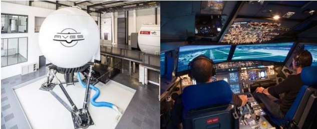
Fig. 12 The motion-based AVES A320 research simulator
