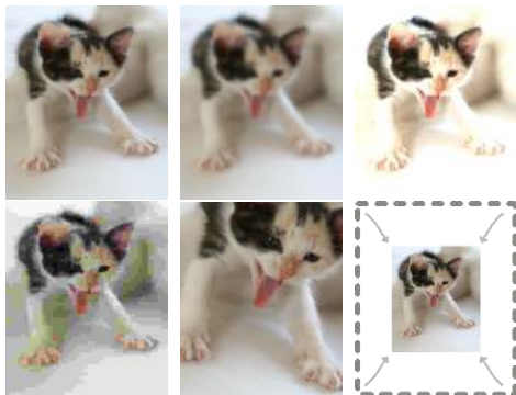
Figure 2: Example of the image perturbations considered. Top to bottom, left to right: original, then blur, illumination, JPEG artefact, rotation, and scale perturbations.
