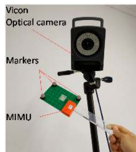
Figure 6. A rigid-body object where both markers and MIMU are attached.
