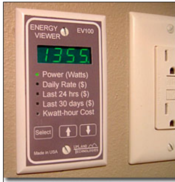
Figure 1. Wall-mounted display of Energy Viewer feedback device.
