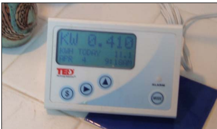
Figure 3. Free standing display of The Energy Detective (TED) feedback device.
