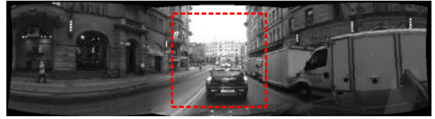
Fig. 3. Illustration of the images captured by the on-board camera in dataset A. The dashed box indicate the central area used for all experiments (except for Wide-GIST results in Fig. 9 that are based on the full image).
