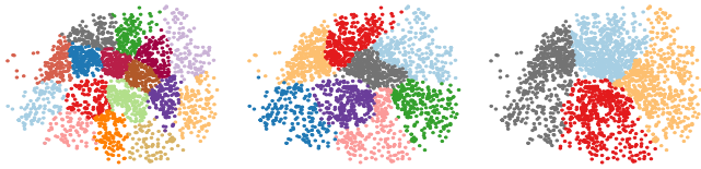
Figure 8: Association of antenna sites to level- \ell nodes in the large metropolitan scenario. The plots refer to \ell = 8 (16 nodes, left), \ell = 9 (8 nodes, middle) and \ell = 10 (4 nodes, right). Figure best viewed in colours.
