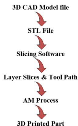
Figure 2. Generalized AM process steps
