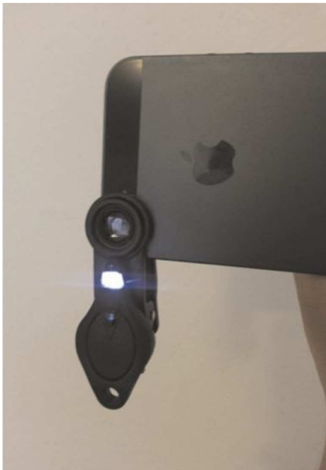
Figure 5. Smartphone adapter for anterior segment imaging developed by Myung et al.
