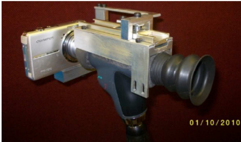
Figure 6. Panoptic monocular indirect ophthalmoscope (Welch-Allyn Inc., Skaneateles Falls, NY, USA) customised so to capture images with a wireless enabled digital camera. A cellphone then received these images for long-distance transmission.
