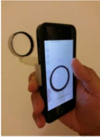
Figure 4. The '3D Printed Smartphone Indirect Lens Adapter' developed by Myung et al. consists of a condensing lens held at a fixed length from the Smartphone's camera by a 3d printed adapter.
