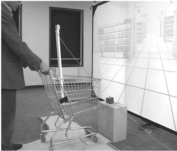
Figure 3. Behavioural interface using a trolley fitted with instruments for moving in a virtual store (photo Mines ParisTech)
