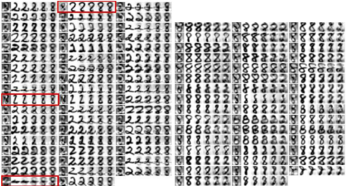
Figure 4: USPS digits (training set): “twos” (left) and “eights” (right) with correct classification. For each digit from left to right: (i) explanation vector (with black being negative, white being positive), (ii) the original digit, (iii-end) artificial digits along the explanation vector towards the other class.
