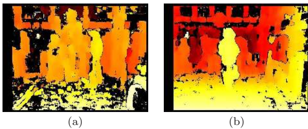
Fig. 16 Disparity maps of two frames. Disparity is coded by using a hot color space representation. In this representation, close 3D points to the camera are depicted in yellow, whereas far points are depicted in red. Best viewed in color.
