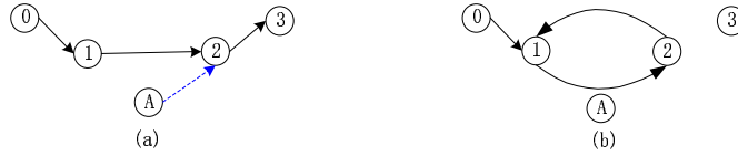
Fig. 2. The attacker forms a loop between node 1 and node 2 by a faked RREP message. (Node 0: originating node; nodes 1 and 2: intermediate nodes; node 3: destination node; node A: attacking node.)
