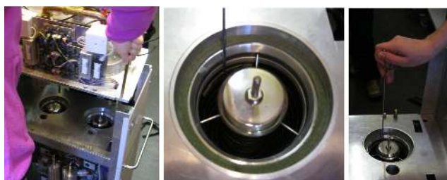
Figure 10. Cleaning electrometer rings by lifting away the sample preconditioning unit (the top part of the NAIS) and using a long cleaning rod to wipe the surface of outer electrode.
