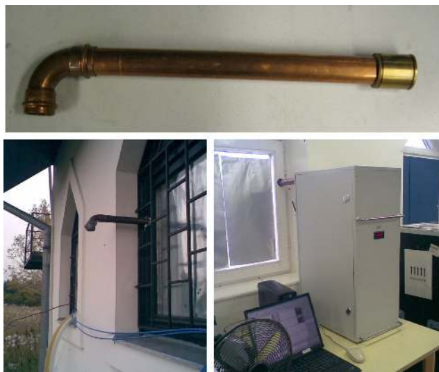
Figure 7. Example an aerosol sampling inlet for the NAIS used at K-pusztá field station, Hungary. A grid is missing in the top image from the end of the sampling line. Below an instrument set-up on field.
