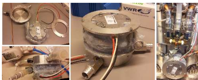
Figure 15. Procedure for replacing a blower for a 1-blower instrument.
