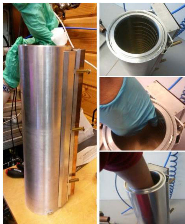
Figure 11. Cleaning electrometer rings by opening the mobility analyzer and wiping with a clean cloth.
