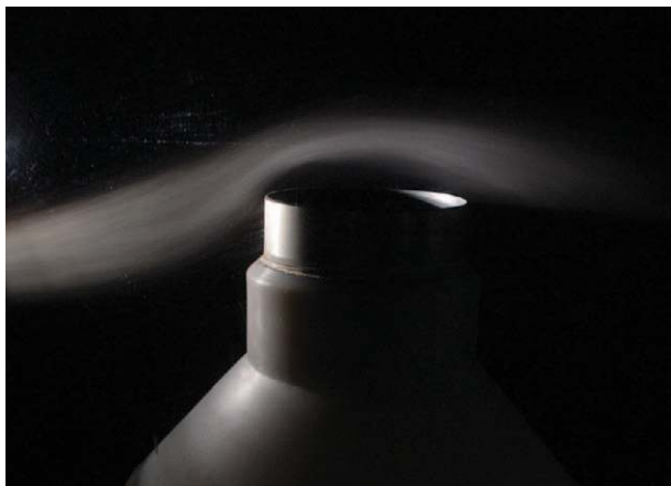
FIG. 17. Mapping of airflow around a gauge orifice in laminar wind tunnel flow.
