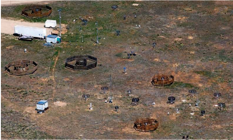
FIG. 4. Aerial view of the Marshall Field Site. The three large shields with two concentric fences in the top left are full-size DFIR shields, and the two small DFIR (SDFIR) shields in the foreground with two concentric fences are two-thirds the size of the DFIR shields. At the center of each SDFIR is located a single Alter shield with a GEONOR snow gauge. Smaller single and double Alter shields are located at various locations at the site. Vegetation is less than 0.25 m tall.
