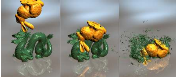
Figure 2: These images are from the breaking dragon benchmark consisting of 252 K triangles, the most challenging benchmark in our test sets. Our method spends 54 ms for CCD including self-collisions and achieves 12.5 times improvement over a serial CPU-based method.
