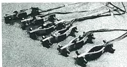
Fig. 18. Special strain gage units, each containing four SR-4 gages encased in small blocks of concrete mortar after calibration.
