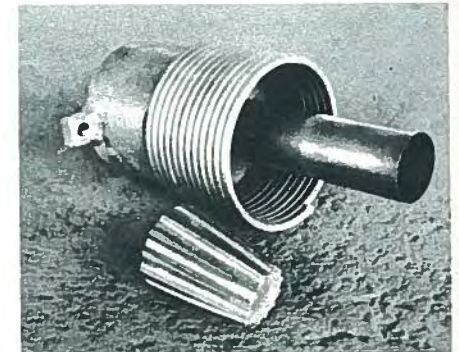
Fig. 60. Forged steel socket and fluted aluminum plug. The relatively soft aluminum plug deforms during stressing and becomes "keyed" to the wire tendons. Since the wires themselves do not deform, there is little tendency to weaken the wires at the grip.
