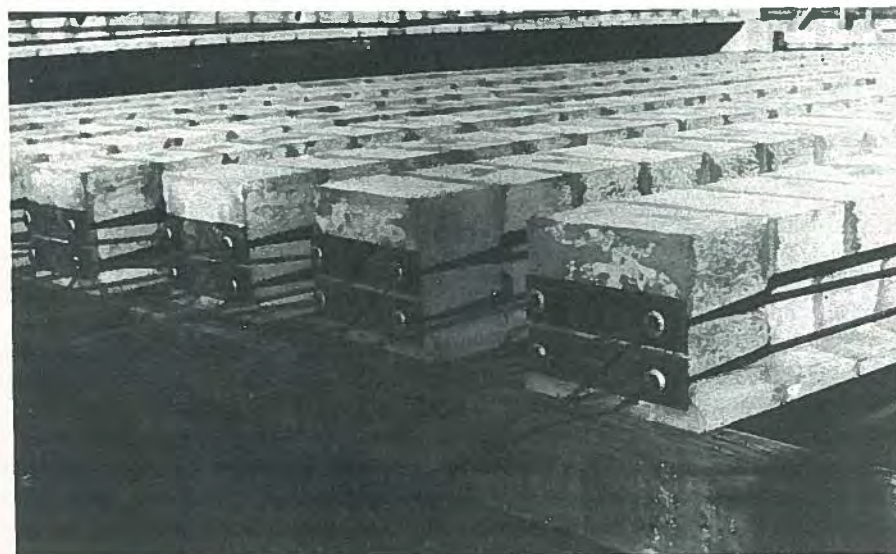
Fig. 9. A 16-in. (406 mm) bridge beam with bonded strands.
