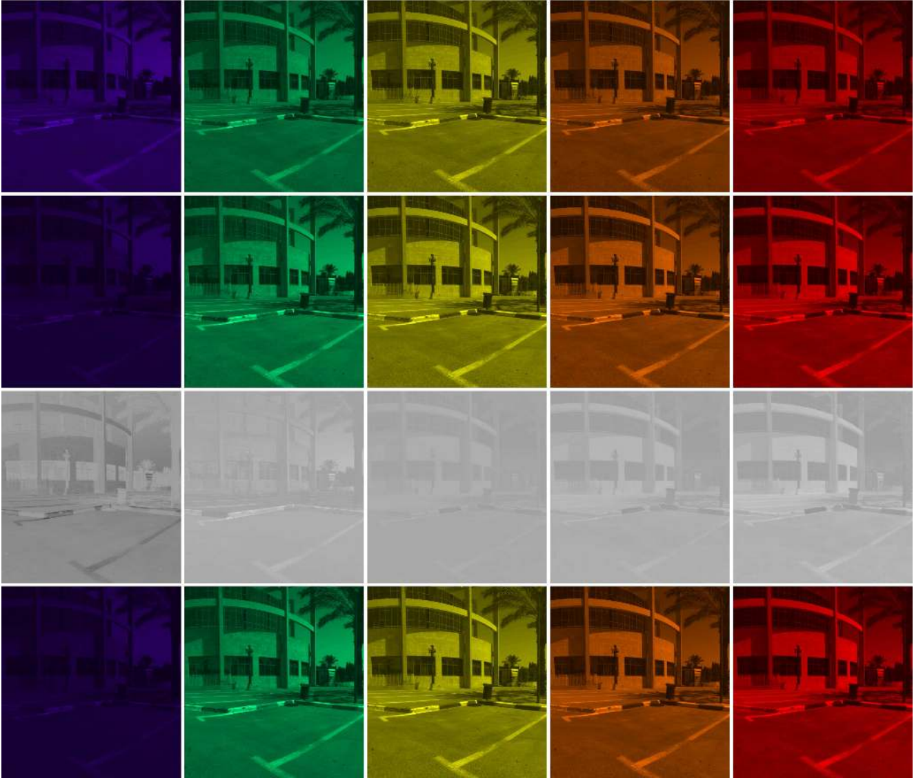
Figure 3. Visual results of five selected bands for RGB to hyperspectral conversion. From top to bottom: interpolation, HSCNN, residuals learned by HSCNN (properly scaled for better visualization), and groundtruth. From left to right: 430nm, 500nm, 570nm, 600nm, 630nm.
