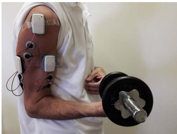
Fig. 6 Recording setup. Photograph of the recording setup with the wireless electromyograph sensors worn on the upper right arm with their electrodes placed on the biceps brachii , deltoideus medius , and triceps brachii muscles
