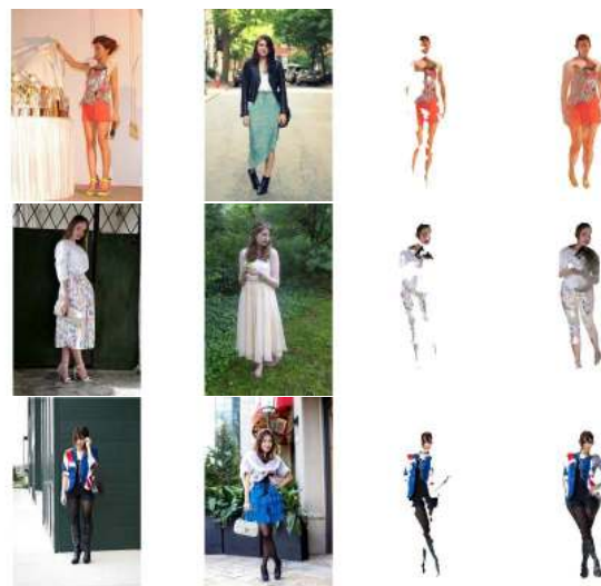
Figure 9. Sample results for the body color completion module. From left to right: source image, target image, appearance data copied using visible mesh triangles on both meshes (source and target), appearance data completed using vertex color completion.
