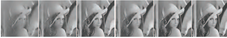
Fig. 11. Illustration of the distortions introduced by general compression methods (three first images on the left) compared to saliency-based compression (three last images on the right), at three different compression levels. Adapted from Yu & Lisin (2009))
