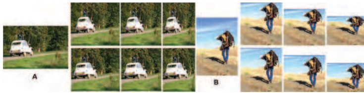
Fig. 17. The original images (A and B) and for each one seams removal (vertical seams for A and horizontal seams for B) using gradient (top-row) and using a saliency map (bottom row). Adapted from: http://cilabs.kaist.ac.kr
