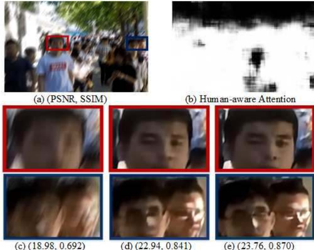
Figure 5: Demonstration of attention module for deblurring. (a) Blurred image. (b) Attention mask. (c) Blurred details. (d) Deblurred w/o attention. (e) Deblurred w/ attention. See §5.1.
