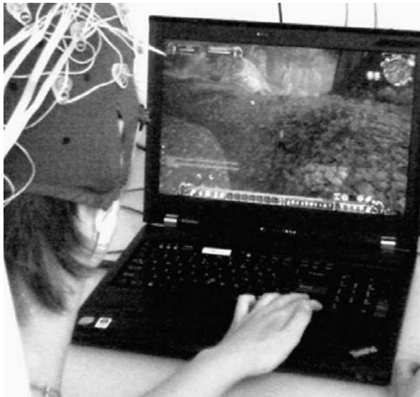
Figure 3. A user playing World of Warcraft® with both conventional controls and mental states to control the character in the game [8]. World of Warcraft® is a registered trademark of Blizzard Entertainment.
